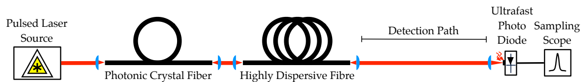
Figure 1: Scheme of the experimental setup of the single-shot spectrometer. A pulsed fiber laser pumps the supercontinuum generation in the PCF. The high dispersion in the next module leads to a separation of reddish and blueish wavelengths in time enabling broadband spectral measurements with ultrafast temporal sampling methods.
