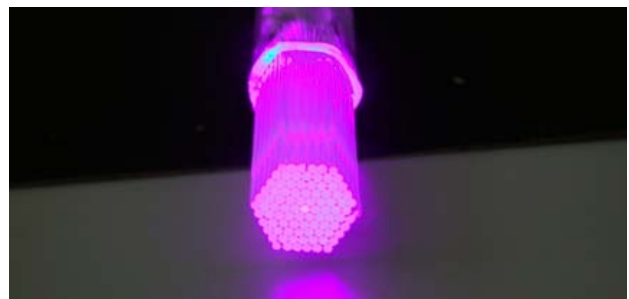
Figure 2: Stacked fiber preform with doped core.
