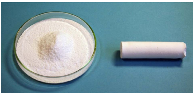
Figure 1: Doped powder and the resulting green body.
